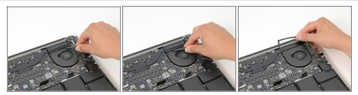
• In the same manner described above, release the adhesive and flip back the heat sink cover on the left fan.
